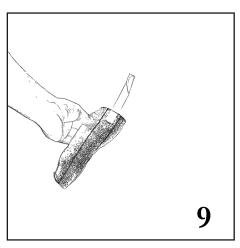
Then you can apply the tape on one end of the wick. Double it precisely so the tape won't stick inside the burner.
