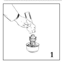
Remove the glass chimney and check for dead bugs and dirt which can block air supply.
