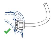
Include cable slack at the entering point of the cable gland
