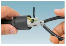
3. Cut off the stranded wire ends so they are flush.
